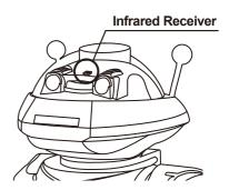
CAUTION: To operate it at its best, the controller should be aiming at the receiver on the robot's head
