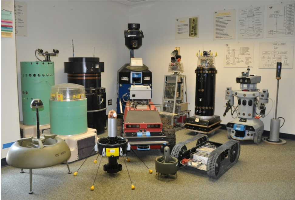
Figure 2. Ground robots in the museum area of Building 624 (left to right across the back wall) include two ModBots , A Denning Sentry , an MDARS-Interior security robot, ROBERT I , ROBERT II , and ROBERT III . An iRobot All Terrain Robotic Vehicle is at image center, with the original prototype of the URBOT at lower right. A few prototype ducted-fan air vehicles are at foreground left.
