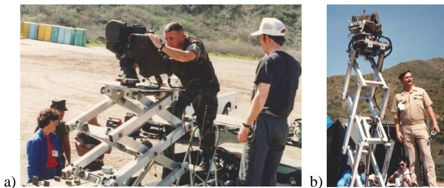
Figure 123. a) Robin Laird (right) and Gunnery Sargent Burke (center) boresight the MULE laser designator on the Surveillance Module at Camp Pendleton, CA, while Celia Metz (lower left) confers with Major McNamee and Captain Murray. b) Commander Everett supervises subsequent MULE testing with the mast fully extended.
