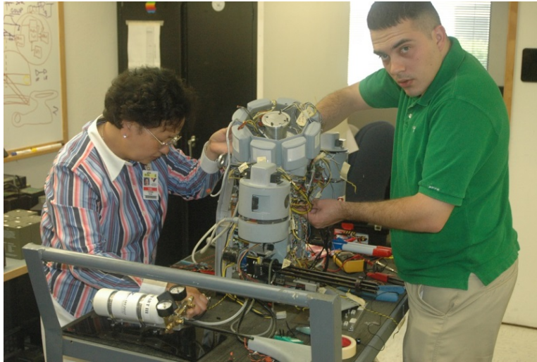
Figure 180. Electronics technician Yuong Sun (left) and electrical engineer Brandon Sights (right) reassemble ROBART III following extensive reconfiguration to accommodate the new 16-bit torso computer in 2006.
