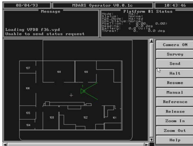
Figure 167. An Operator Station could be automatically assigned to any specific robot when the detailed attention of a guard was required, allowing the supervisor to allocate both computational and human resources in response to exceptional events (Everett, Heath-Pastore, & Hower, 1994).
