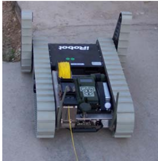
Figure 245. One of four iRobot PackBot Explorers equipped with the CHARS payload. Note iRobot 's fiber-optic spooler for improved communications when entering caves and bunkers.
