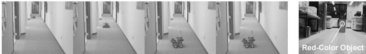
Figure 235. The Pioneer AT test surrogate enters the hallway (far left), traverses past Room 360, turns towards the copy room (center), and comes to a halt upon detecting the target object in the copy room (far right) (images adapted from Arkin, Collins, & Endo, 1999).
