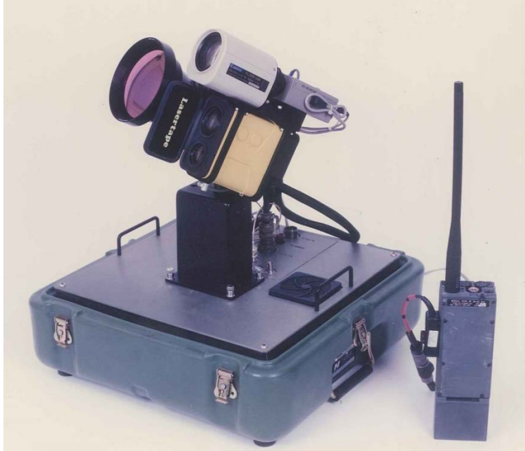
Figure 217. The ground-based MPP sensor package included both visible-light and infrared video cameras, a laser rangefinder, and an optional acoustic sensor collectively mounted on a commercially available pan-and-tilt unit.
