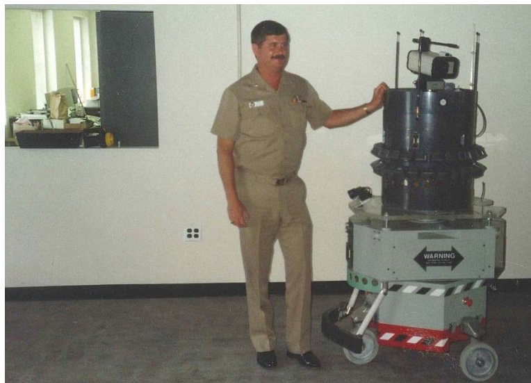
Figure 144. Shown here atop a Cybermotion K-2A Navmaster mobility base, the ARDEC MDARS-Interior payload was a 24-inch-diameter ModBot configuration with six stacked modules for video, acoustic, microwave, passive infrared, sonar, and security assessment.
