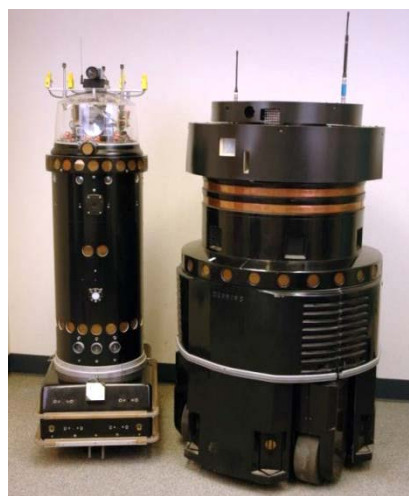
Figure 159. Shown here next to ROBART II in the museum area of Building 624 Seaside, the Denning Sentry employed microwave and passive-infrared motion sensors similar to those used on ROBART II . Denning began development of the Sentry in August 1983 (Everett, 1998).
