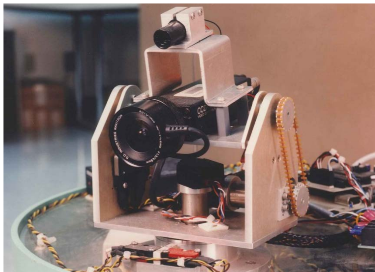
Figure 223. A laser pointer was added to the camera pan-and-tilt unit of the ModBot by Hoa Nguyen. This configuration was eventually replaced by the stereo Zebra Vergence system offered by Transitions Research Corporation (TRC), Danbury, CN, shown later in Figure 225.
