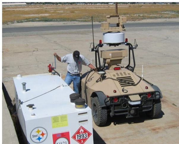
Figure 206. Jack Gonzales refuels the MDARS-Exterior robot during Early User Appraisal at Hawthorne, the world's largest army depot (147,000 acres), circa 2005.
