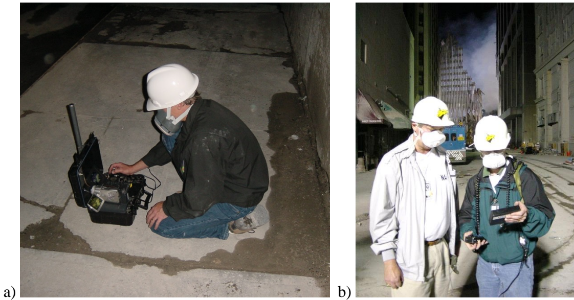
Figure 240. a) Robin Laird controls the Foster-Miller Special Operations Lemming (SOLEM) robot from its compact self-contained operator control unit. b) Mike Bruch (right) controls one of three URBOTs while Bart Everett looks on, with the remains of WTC Tower Two in background.
