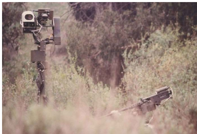
Figure 121. The TOV concept allowed RSTA missions to be carried out from a vehicle in defilade, with a 0.50-caliber Weapon Module for self-protection (lower right). Validated targets were illuminated by the MULE laser designator atop the Surveillance Module (upper left) for a Hellfire missile or Copperhead projectile strike.
