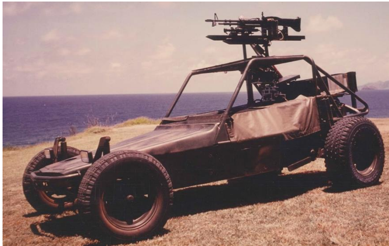
Figure 110. Live-fire exercises demonstrated the ability to position the teleoperated dune buggy at a 2- to 4-kilometer standoff distance with remote pan, tilt, and trigger control of the weapon system. To facilitate aiming, an additional video camera was attached to the M60 gunsight.
