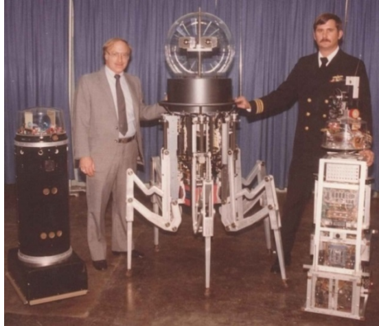
Figure 92. Russ Werneth of NSWC and Lieutenant Commander Bart Everett of SEA-90G with ROBART I , ROBART II , and the Odex robot by Odetics at the NSWC Robotics Lab, circa 1985. Note the six gold Polaroid electrostatic sonar transducers on ROBART II , versus the single black piezoelectric transducer on ROBART I .
