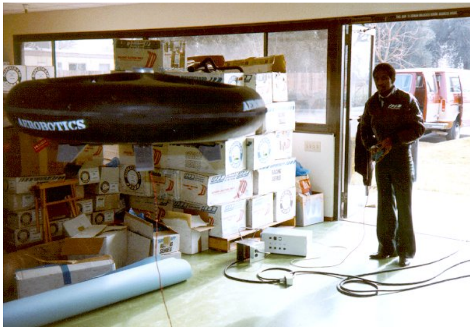
Figure 12. The tethered Airborne Remotely Operated Device (AROD) was an electrically powered quadrotor developed by Moller International and tested as an airborne remote-presence system at the NOSC HI Lab.
