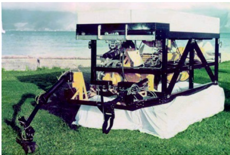
Figure 69. Shown here at the NOSC Hawaii Laboratory on Kaneohe Marine Corps Air Station, Oahu, the Remote Unmanned Work System (RUWS) Work Vehicle measured 4.5 by 4.5 by 11 feet long, weighed 4300 pounds in air, and could operate down to 20,000 feet (Talkington, 1978).
