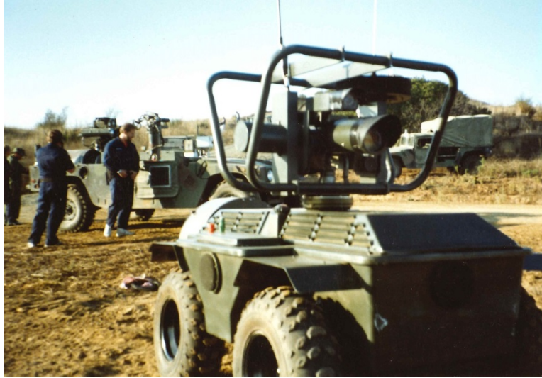
Figure 127. The Martin-Marietta TMAP (foreground) participated in the 1989 “Tele-Robotic Vehicle Demonstrations” (see also Figure 128), along with the Grumman TMAP (not shown) and the NOSC TOV (background left). The fiber-optic cable-recovery vehicle developed by Code 531 is at background right.
