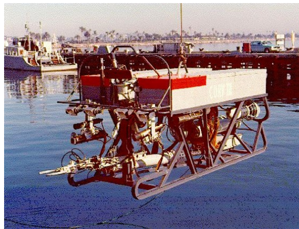
Figure 72. After recovering wreckage from the Space Shuttle Challenger disaster in January 1986, CURV III was transferred to the Navy Supervisor of Salvage (SUPSALV) and upgraded for operations down to 20,000 feet. The rugged and enduring unmanned undersea system was still operational almost 30 years later.
