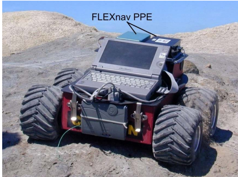
Figure 232. The University of Michigan's FLEXnav PPE precision dead-reckoning system implemented on a Pioneer AT .
