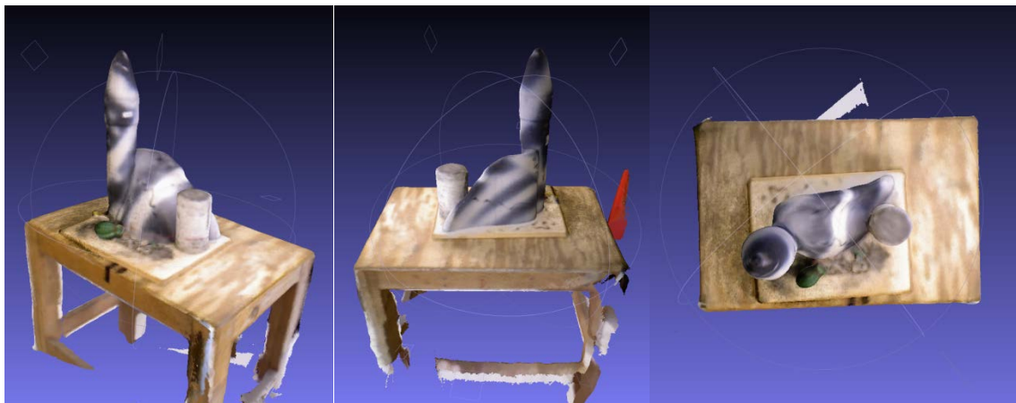
Figure 46. Created by stitching successive video frames together in 2 minutes or less, this 3D model of a training IED could be viewed by the UGV operator from any desired perspective for detailed near-real-time analysis.
