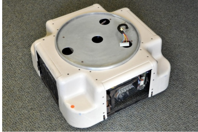
Figure 140. Manufactured by Transitions Research Corporation, Bethel, CN, the LabMate was used as a mobility base by a number of research groups, and formed the basis of the company's later HelpMate robot (Katevas, 2001). The circular aluminum base plate accepts the stacked-ring ModBot payloads shown in Figure 141.
