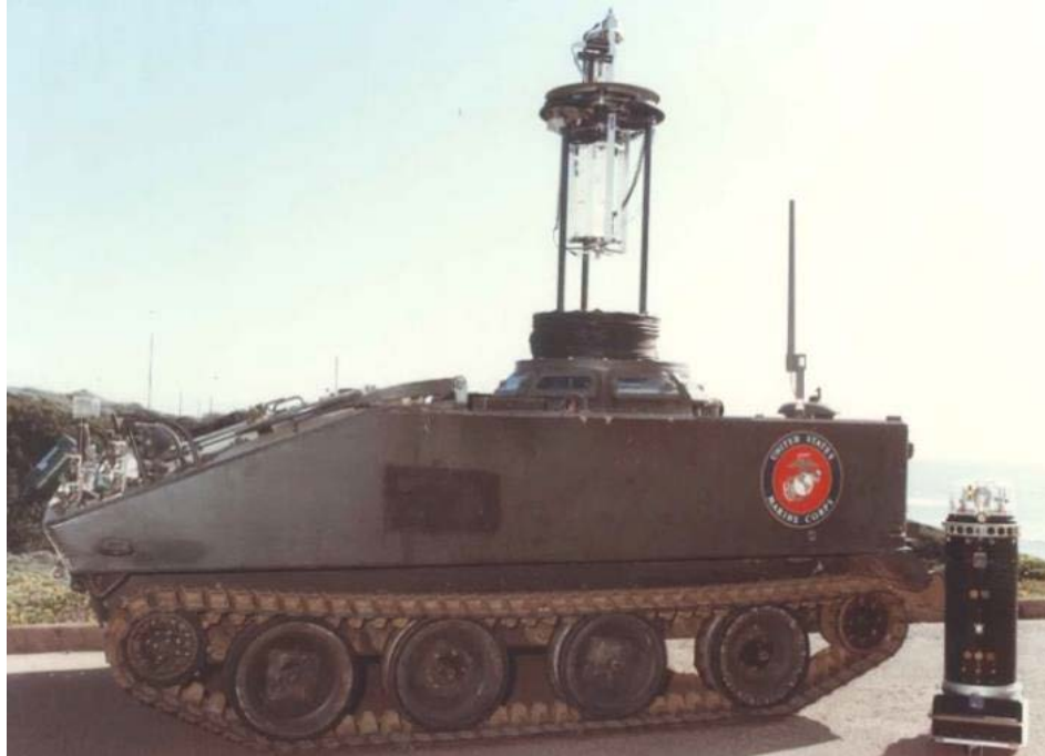
Figure 8. The Code 442 autonomous Ground Surveillance Robot (GSR) was based upon an M-114 Command and Reconnaissance Carrier . At right is ROBART II , newly arrived from Springfield, VA, circa December 1986.
