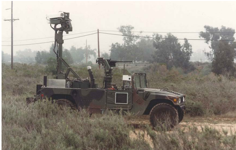
Figure 117. TOV-1 undergoes field testing by Code 535 at the Marine Corps Tactical Systems Support Activity (MCTSSA), Camp Pendleton, CA, in 1988. The TOV operator was provided with stereo head-coupled visual displays, binaural audio, and driving controls isomorphic to those found in a HMMWV (Aviles et al., 1990).
