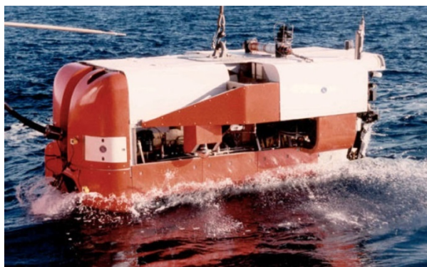
Figure 137. The steel lift line is attached to the lifting ring (top center) of this later ATV configuration, while the power and communications tether is shown at far left. In addition to its four video cameras, the ATV also employed obstacle-avoidance sonar and continuous-transmission frequency-modulated (CTFM) sonar for target acquisition.
