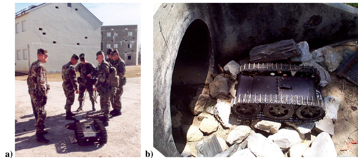
Figure 237. a) Soldiers prepare to lower an URBOT down a manhole at the Fort Drum Military Operations in Urban Terrain (MOUT) site with specially designed tackle that facilitated post-mission asset recovery. b) The URBOT is about to enter this underground culvert on a counter-IED training mission at Fort Polk, LA.
