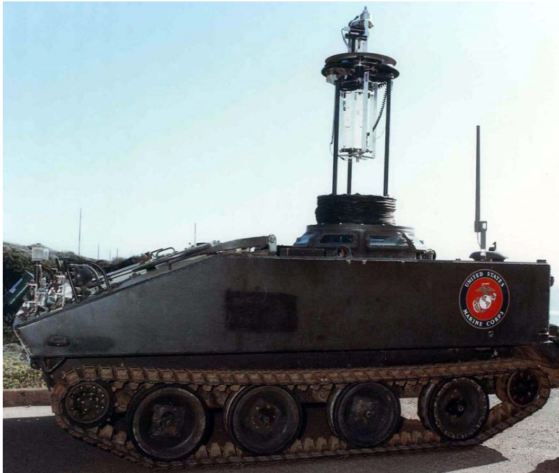
Figure 38. The Ground Surveillance Robot (GSR) was a surplus M-114 Command and Reconnaissance Carrier outfitted by Code 442 to serve as a surrogate testbed for autonomous navigation and collision avoidance, circa 1986.
