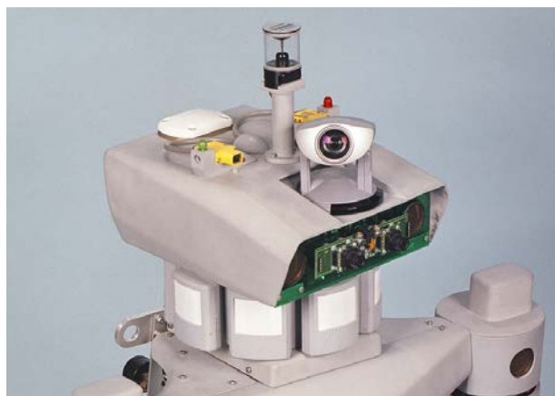
Figure 185. The head-mounted high-resolution PTZ camera was cued to the location of any suspected disturbance sensed by the 360-degree motion-detection sensors (eight passive-infrared detectors around the neck, the Visual Stone omni-directional camera at top center, and a microwave motion detector behind the face plate).
