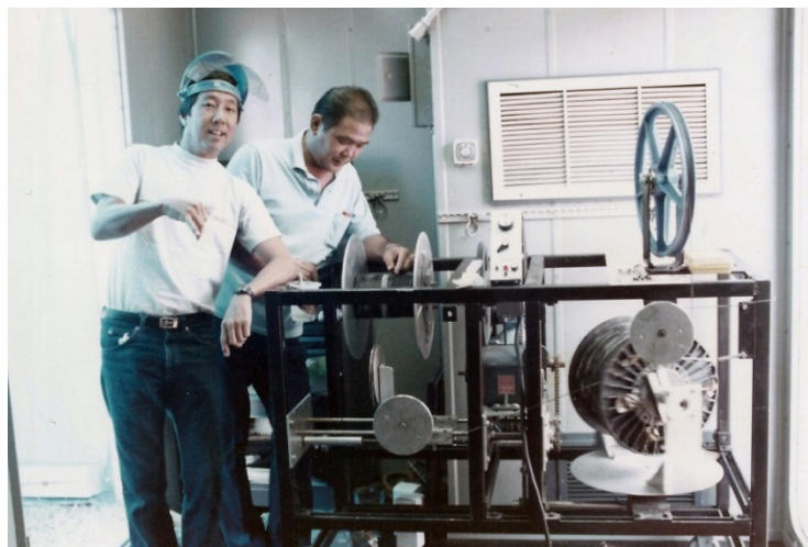
Figure 14. Warren Hahn and Clifford Horikawa of the NOSC Hawaii Laboratory prepare a new spool of fiber-optic cable (image center) with a custom designed winding machine for this purpose. Effective cable winding, payout, and recovery were essential for reliable teleoperation in the field.
