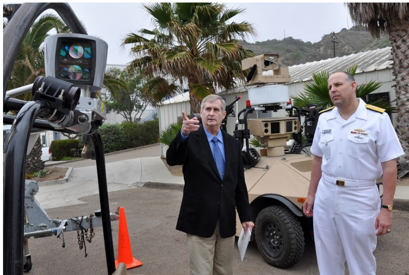
Figure 32. Bart Everett briefs prospective SPAWAR Commander Rear Admiral Patrick Brady on the commercial 3D stereo-camera pair and Velodyne 64 lidar employed on the six-wheel MAX ATV (left), in contrast with the massive custom-built counterpart used on the earlier MDARS-Exterior vehicle in background.
