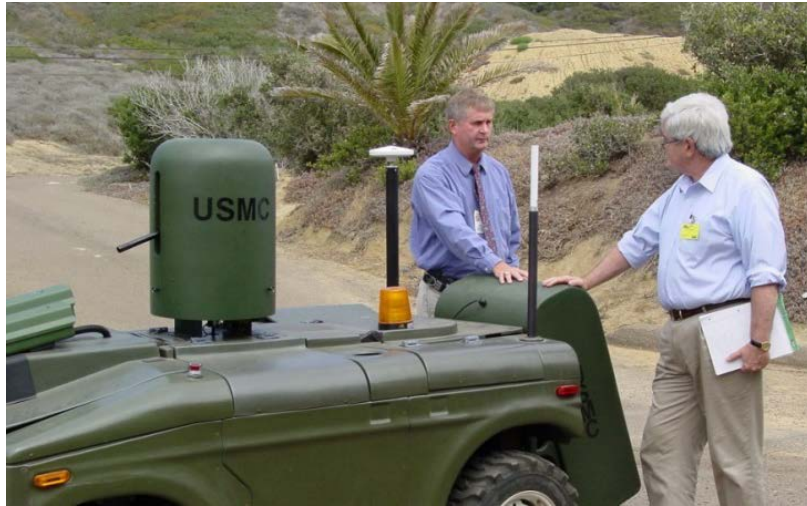
Figure 20. Bart Everett explains the MDARS (BAA version) less-lethal pepper-ball gun pod (upper left) and rear-mounted UGV marsupial carrier for the man-portable URBOT to Mr. Gingrich in the F-36 parking lot Seaside.
