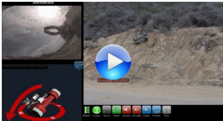
Figure 43. Developed by Aaron Burmeister, Leah Kelly, and Kurt Talke, the tip-over prevention algorithm assesses the various accelerations acting upon the robot relative to its center of gravity (lower left quadrant) as it traverses the slope shown at upper right to detect, warn of, and/or prevent an impending accident.
