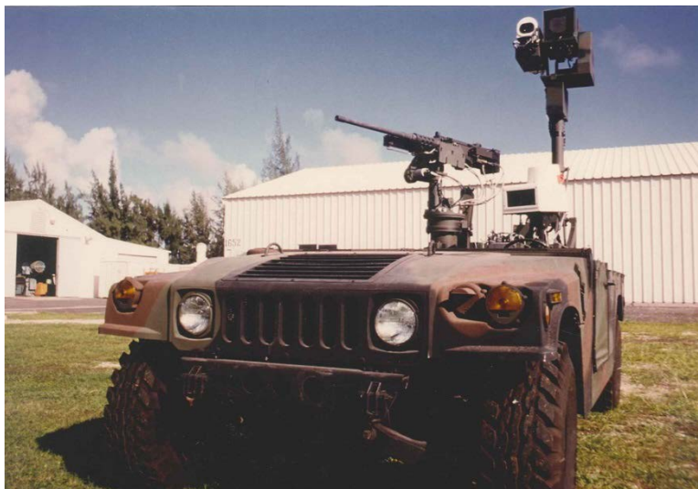
Figure 114. The early Ground/Air TeleRobotic System (GATERS) prototype developed by Code 531 in Hawaii was a remotely driven HMMWV equipped with an elevated reconnaissance, surveillance, and target acquisition (RSTA) payload, with a remotely actuated 0.50-caliber Browning M2 machine gun for self-defense.
