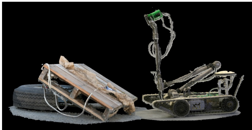
Figure 48. This 3D model of a mock-up suspected IED (left), created from video streams collected by the stereo-camera pair (top), 17 has been merged with an avatar of the iRobot PackBot , which moves in concert with the actual robot to provide the operator with otherwise unobtainable near-real-time situational awareness.
