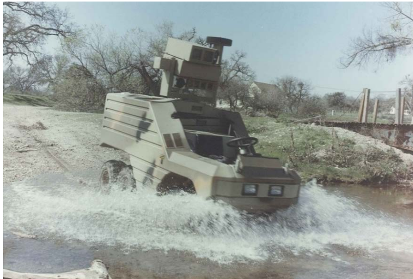
Figure 156. The remotely operated STV fords a shallow stream at Fort Hunter-Liggett, CA, during the Concept of Employment Exercise (COEE) in 1992.
