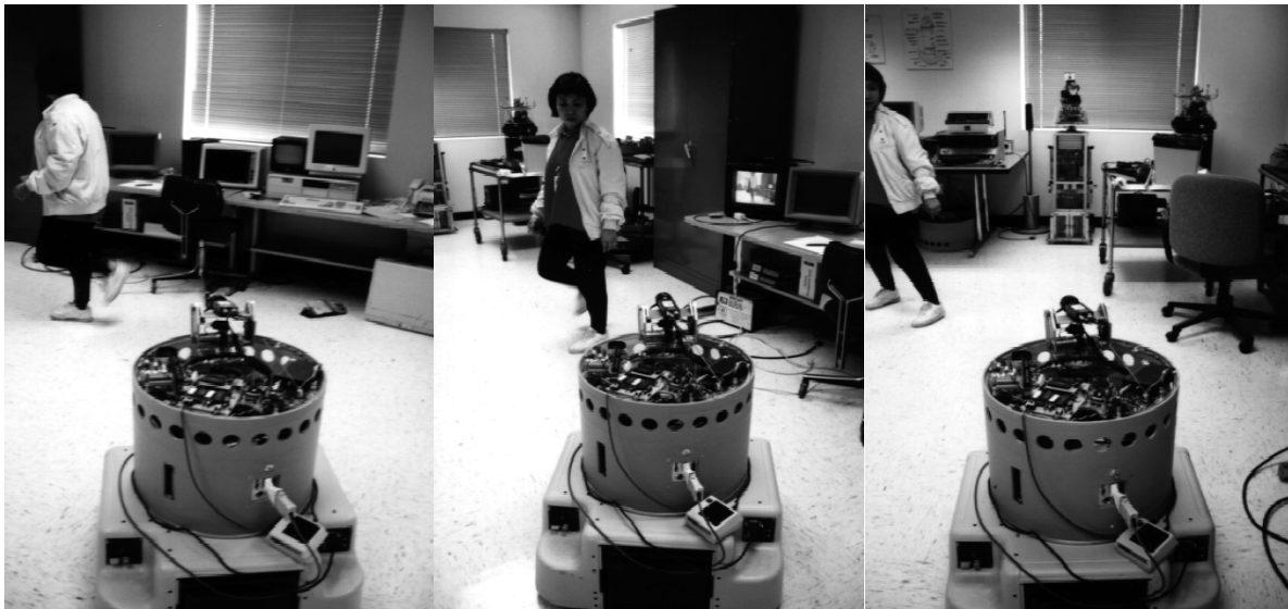
Figure 224. Specifically configured for the Sensor-Motor Transformation project, the visually guided ModBot autonomously trails electrical engineer Theresa Tran as she moves about in Room 115 of Building 622 (adapted from Blackburn & Nguyen, 1994a).
