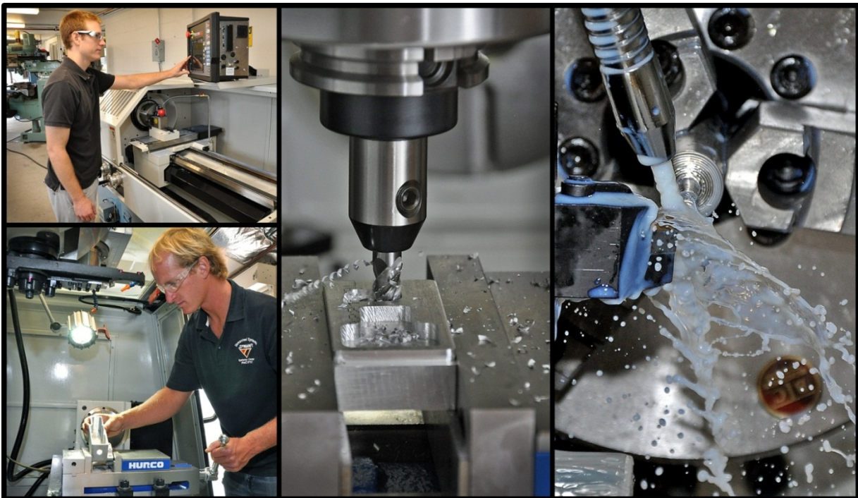
Figure 51: Examples of the new rapid-prototyping equipment in productive use include the Southwestern Industries Trak 1630SX lathe (upper left), Hurco VM10 vertical machining center (bottom left), the VM10 cutting aluminum (center), and the TRAK lathe in action (right).
