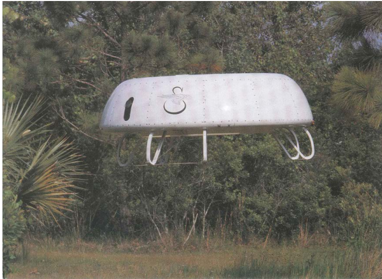
Figure 216. The gasoline-powered Sikorsky Cypher ducted-fan UAV, 6 feet in diameter and weighing some 300 pounds, was selected as the best commercially available VTOL platform for near-term MSSMP demonstrations.
