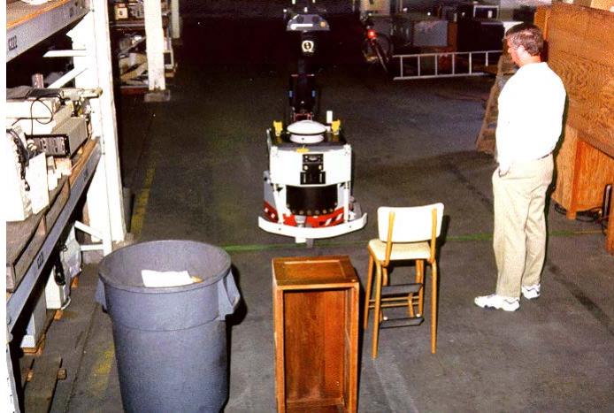
Figure 170. Exhaustive collision-avoidance scenarios were tested during TFT-II to ensure the Cybermotion and NOSC sonar arrays provided proper detection and circumnavigation of all obstacles. The yellow sensors detected retroreflective-tape markers on support columns along the aisle for improved localization (Borenstein, Everett, and Feng, 1996). 43
