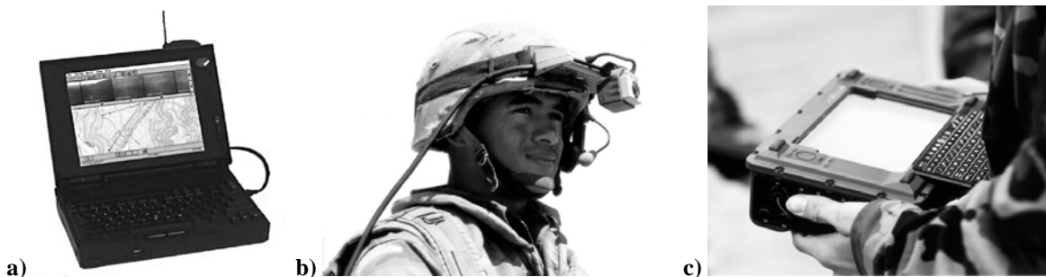
Figure 230. Tested MPNSS control/display configurations included: a) a laptop computer, b) a wearable computer, and c) the Dismounted Soldier System Unit .
