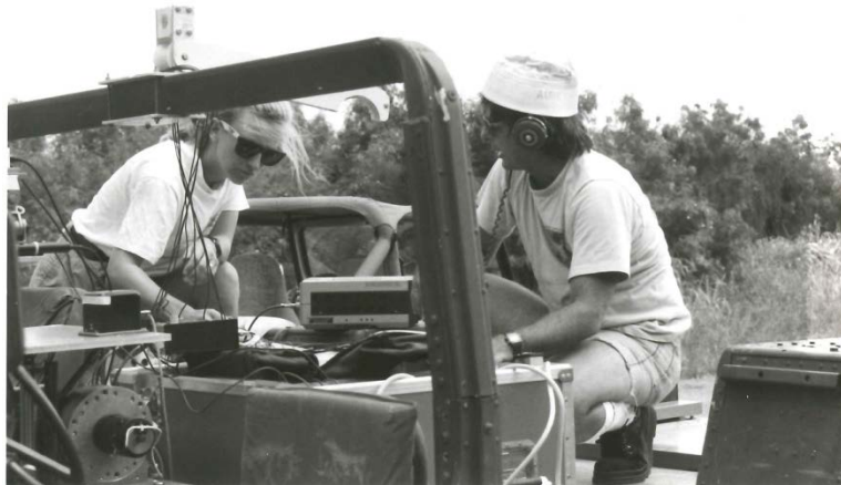
Figure 211. Tracy Heath Pastore (left) and Dr. Jerry Fuqua (right) work on installing the gravity-referenced platform between the HMMWV seats (lower left) at the NOSC HI Lab. Note black 2-DOF inclinometer atop the platform.
