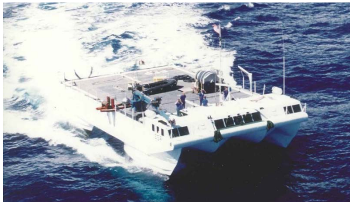
Figure 136. Built in 1973, the NOSC tandem-strut, small-waterplane-area twin-hull (SWATH) vessel SSP Kaimalino provided deployment and recovery services for the ATV undersea vehicle during test and evaluation (Lang & Slogget, 1985). The ATV was designed for operational deployment from a rescue and salvage ship (ARS).
