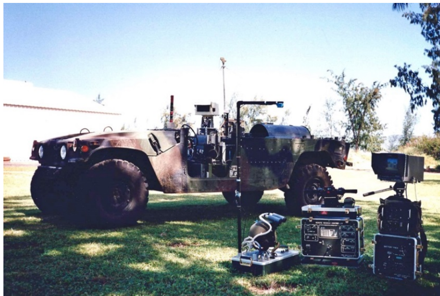
Figure 15. This early version of the GATERS UGV, shown prior to installation of the Surveillance and Weapon Modules, employed a Polhemus 3D tracking system (see blue sensor on L-shaped support above operator's helmet below). The equipment at lower right comprised a portable operator control station.
