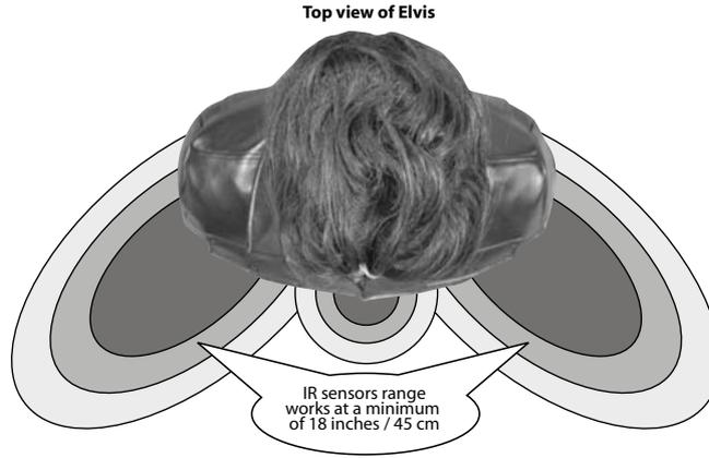
NOTE: Elvis' infrared vision system works at a minimum of 18 inches from his chest. Infrared functions can be affected by bright sunlight, fluorescent and electronically dimmed lighting.
