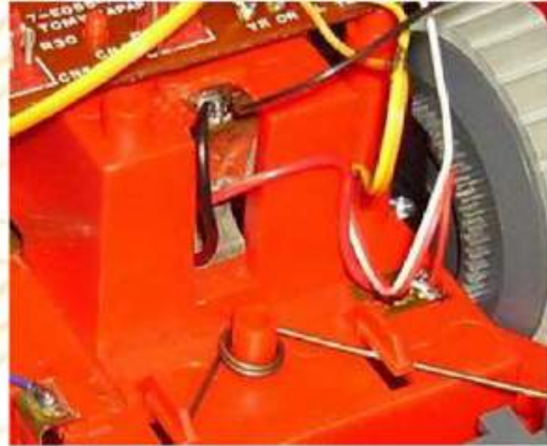
4. Solder the plug and wire to the (+) positive and (-) negative terminals as shown. Click to Enlarge
