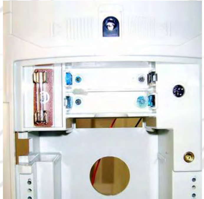
2. Make sure that the batteries are removed from the rear housing.
