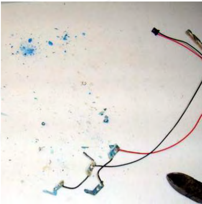
9. This is what the contacts with wire and plug will look like, Replace the battery contacts and solder the wires to the contacts.
