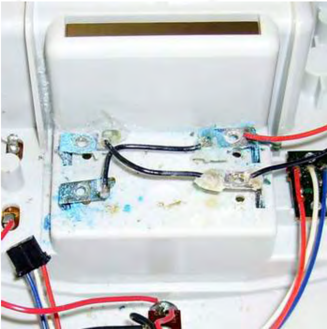
7. Gently pry the battery contacts out.
