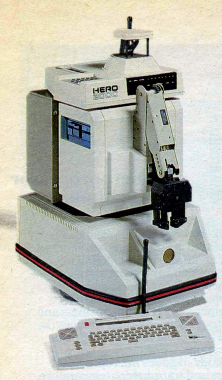
Electronically synthesized voice, temperature and sound sensors are built in
