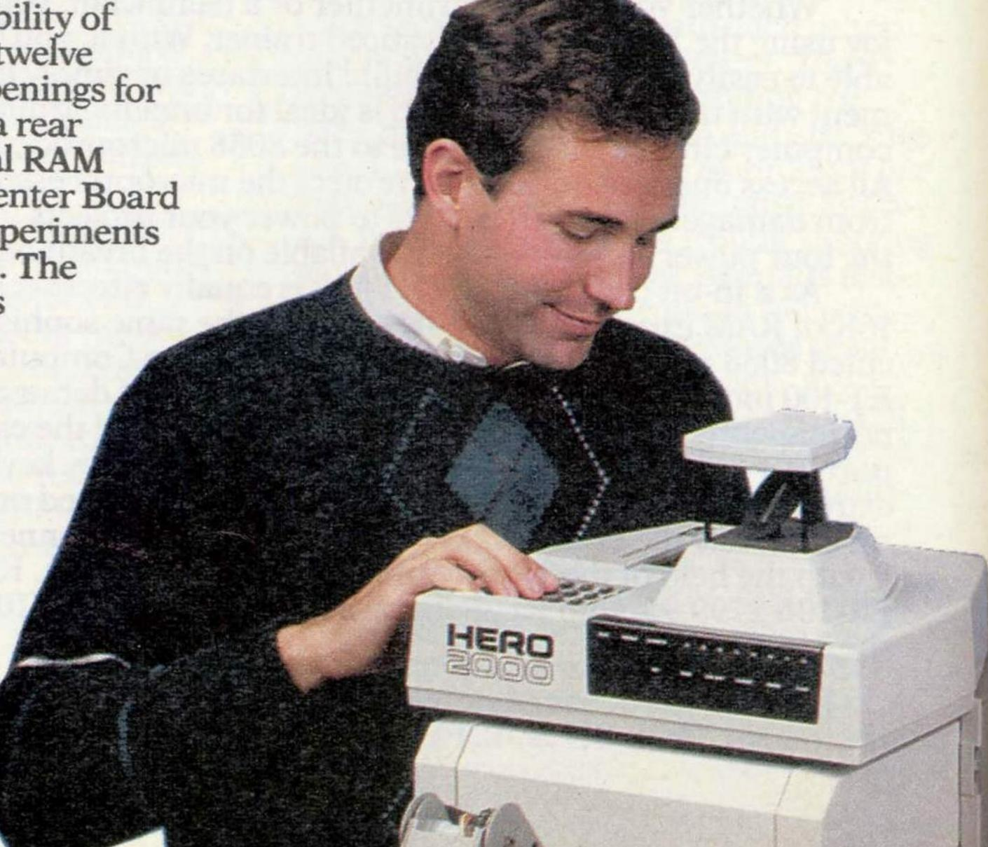
Programming HERO 2000 is done from the top-mounted hexadecimal keypad or the optional wireless remote control (included with an assembled HERO 2000). Sixteen headmounted LED status indicators (eight user definable) show you what function HERO is performing. And with three power modes, HERO 2000 is able to operate from four hours to six days on its single 24 amp-hour battery. A 120 VAC charger is included.
