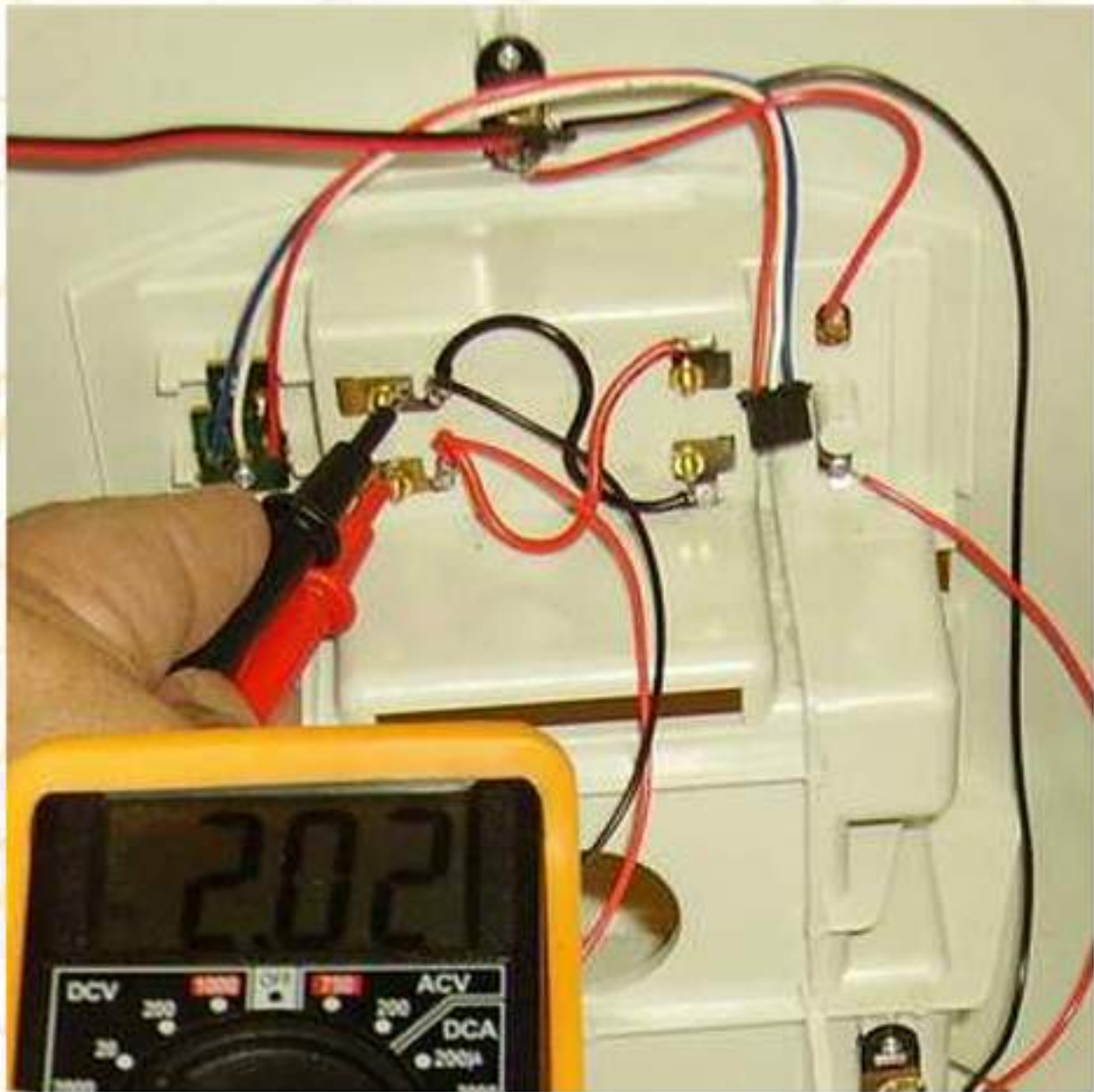
13. Use a multi-meter to check conductivity both at the rear and the plug. Temporary install batteries into the robot housing to check the installation.
