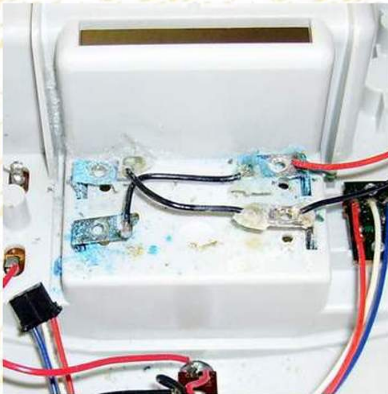
7. Gently pry the battery contacts out.
