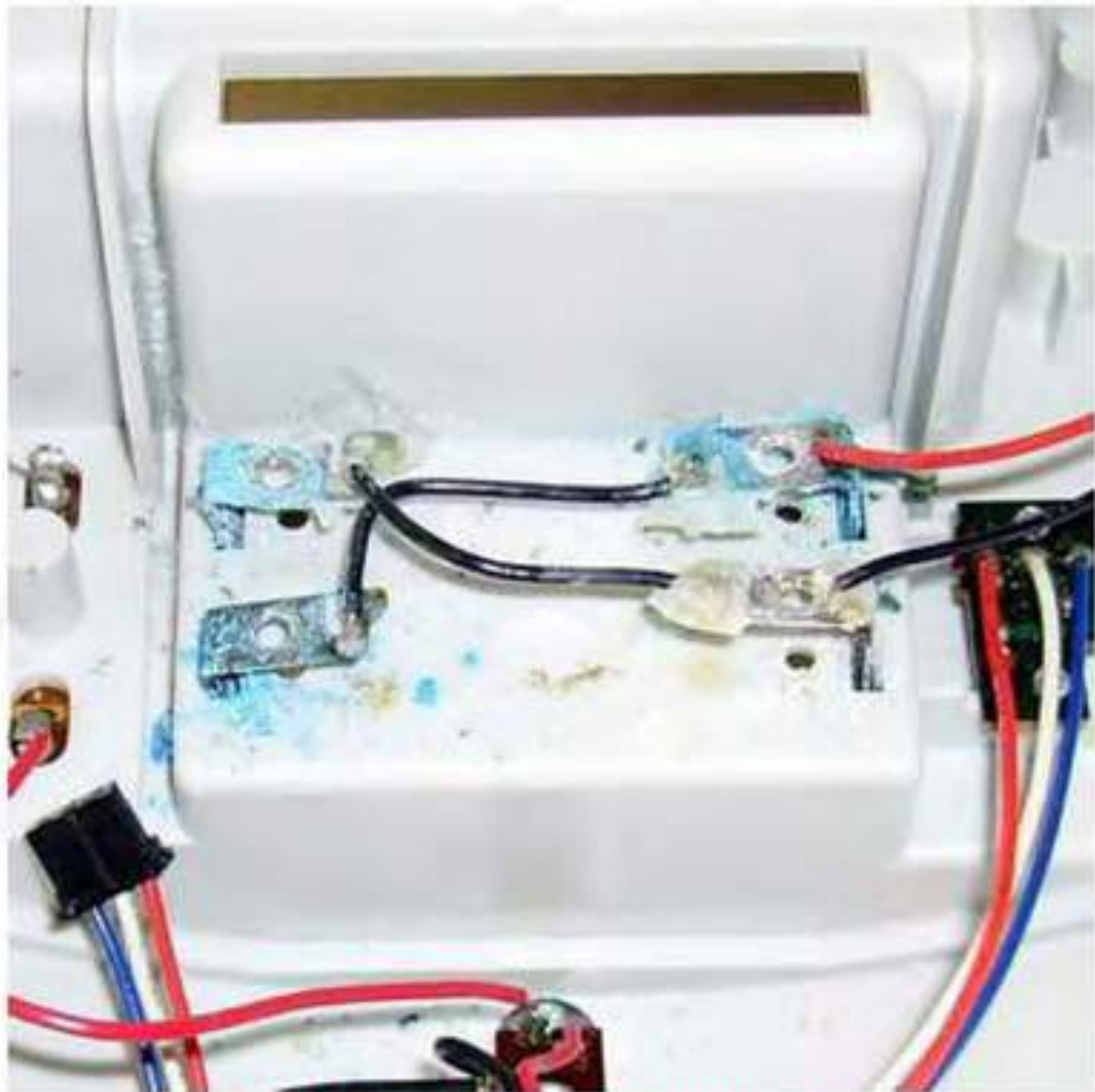
7. Gently pry the battery contacts out.
