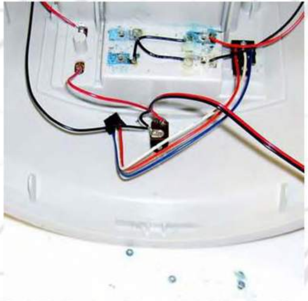
6. This picture shows the eye lit removed from the housing and battery contacts.
