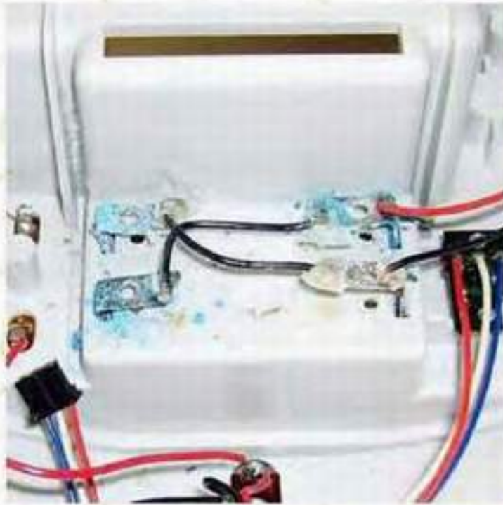
7. Gently pry the battery contacts out.
