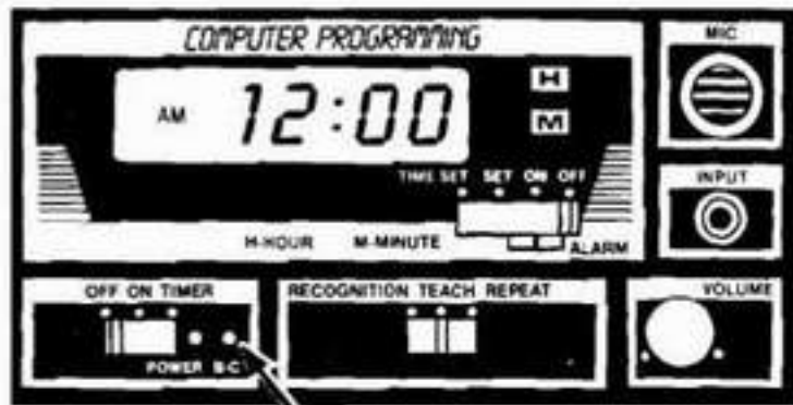
BATTERY CHARGER INDICATOR LIGHT
