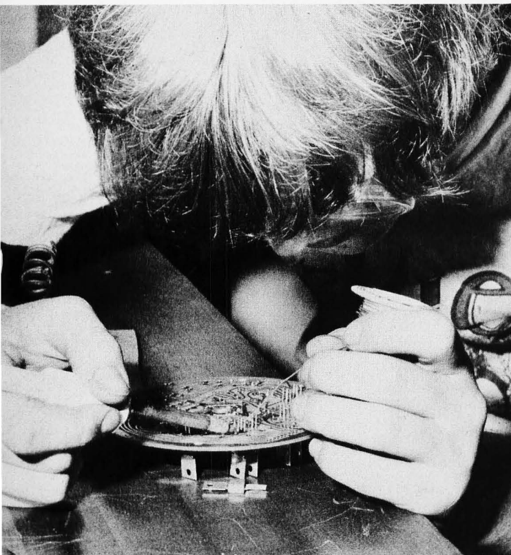
Photo 4: Soldering the installed components.
