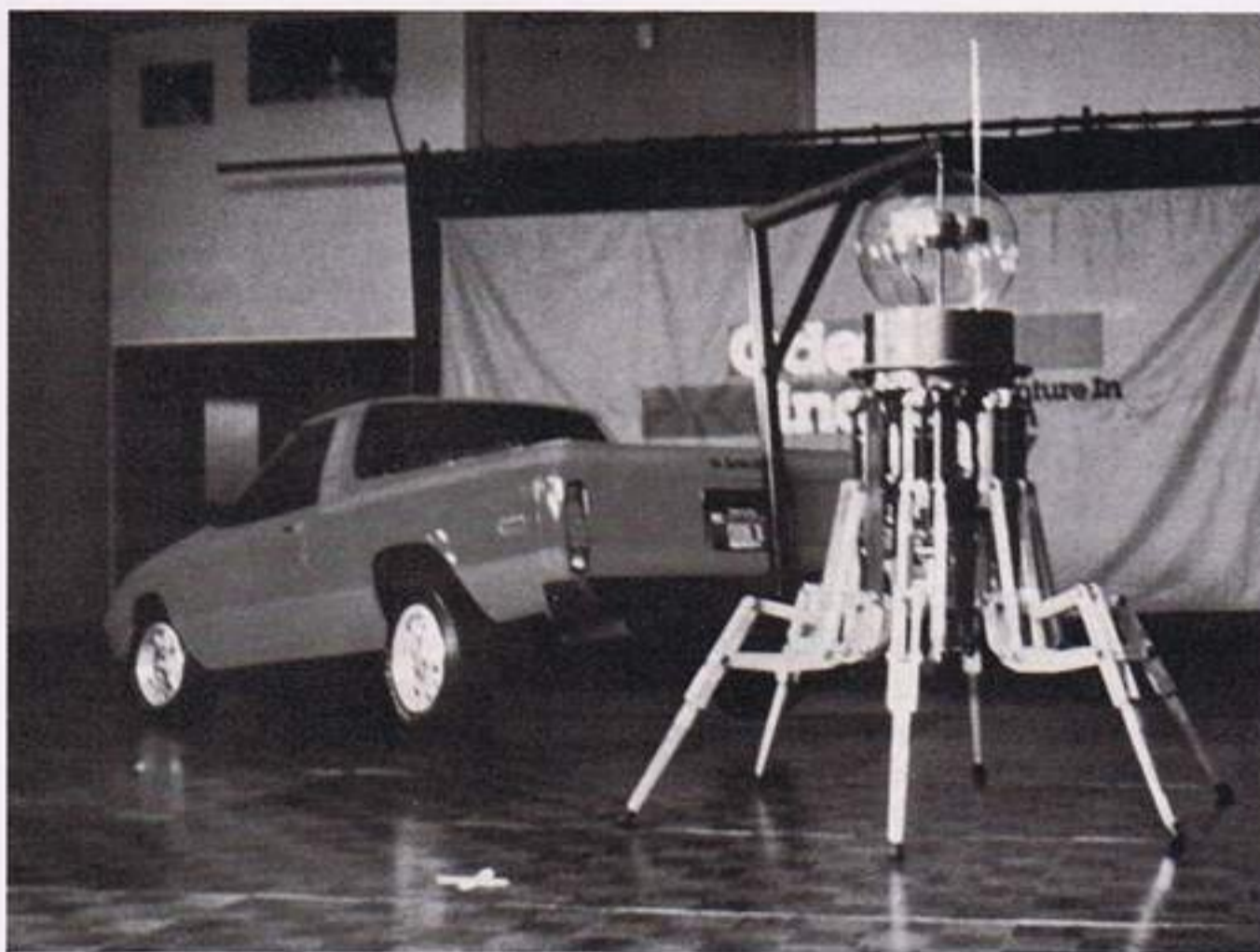
Photo 4. ODEX I walks in the normal profile while lifting the back end of a 2200-pound truck rigged with a special lifting bracket. The first functionoid can lift nearly 900 pounds at normal walking speed, or 2.3 times its own weight.
