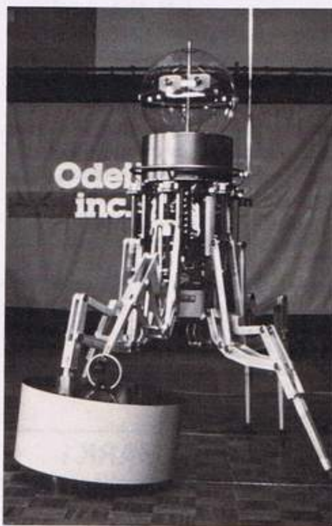
Photo 1. ODEX I executes a feat of agility and strength during the first functionoid's unveiling in Los Angeles last March. In this portion of the demonstration, the unit uses one of its articulators to adjust a swivel ring on top of a pedestal, puts the crutch tip through the ring, then lifts the pedestal. Each articulator can lift as much as 400 pounds.
