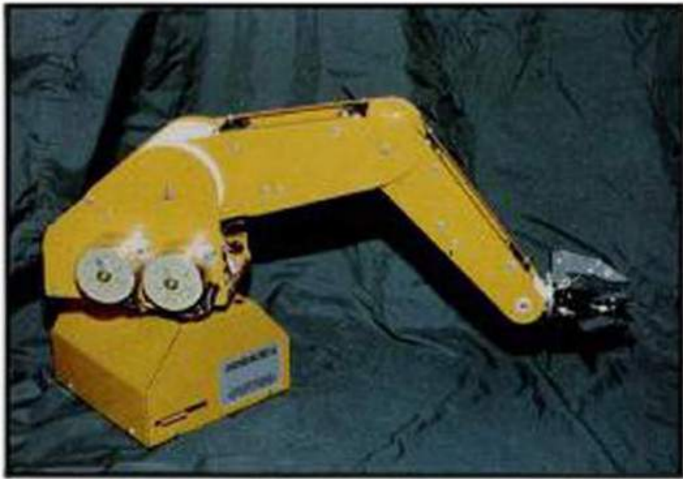
Photo 6: The Armdroid has a maximum reach of 19 inches from the shoulder base.
