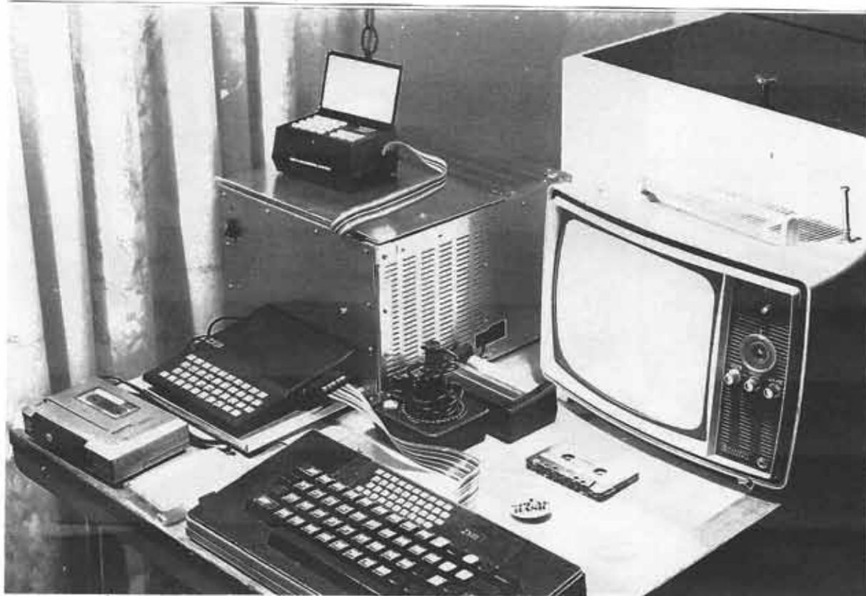
Figure 6-10. Home control center showing computer, external keyboard, expansion and interface boards in enclosure and television monitor.
