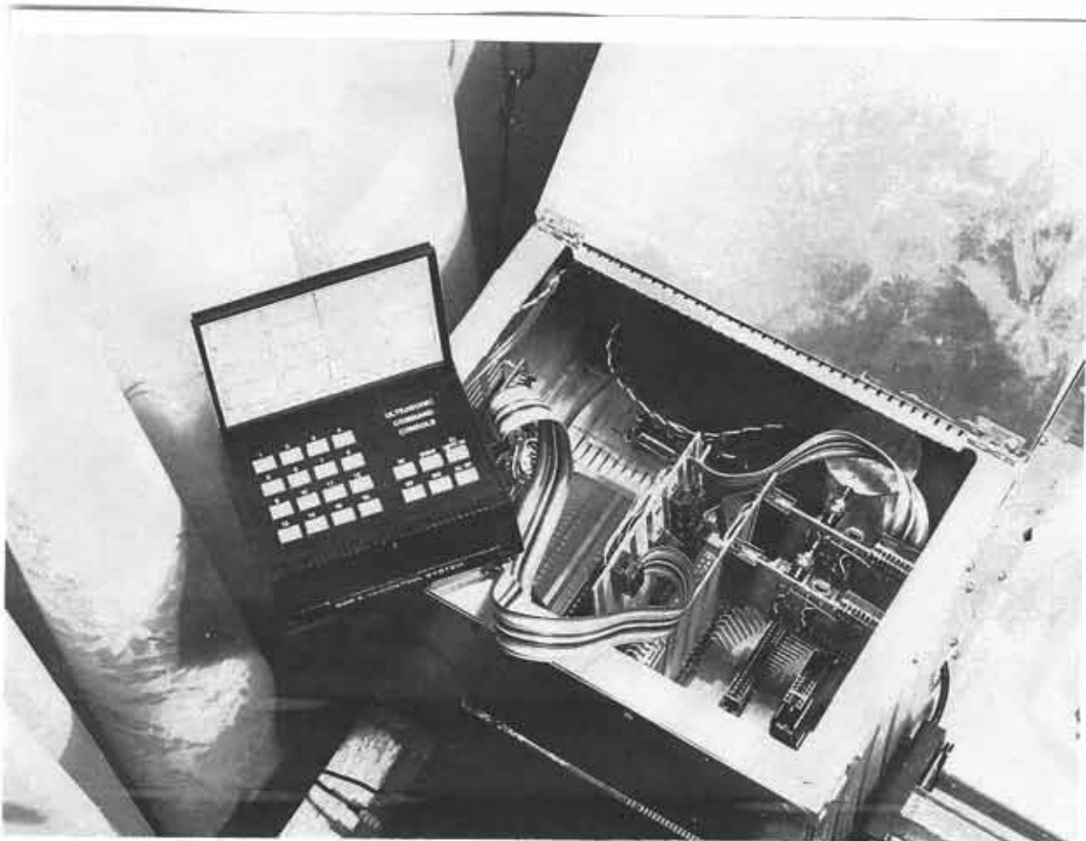
Figure 6-9. Jumper cable shown connecting BSR controller with RX81 board plugged into Expansion Board.
