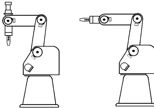
The left image shows the robot with a pitch angle of -90,000. The right image shows the robot with a pitch angle of 0.
