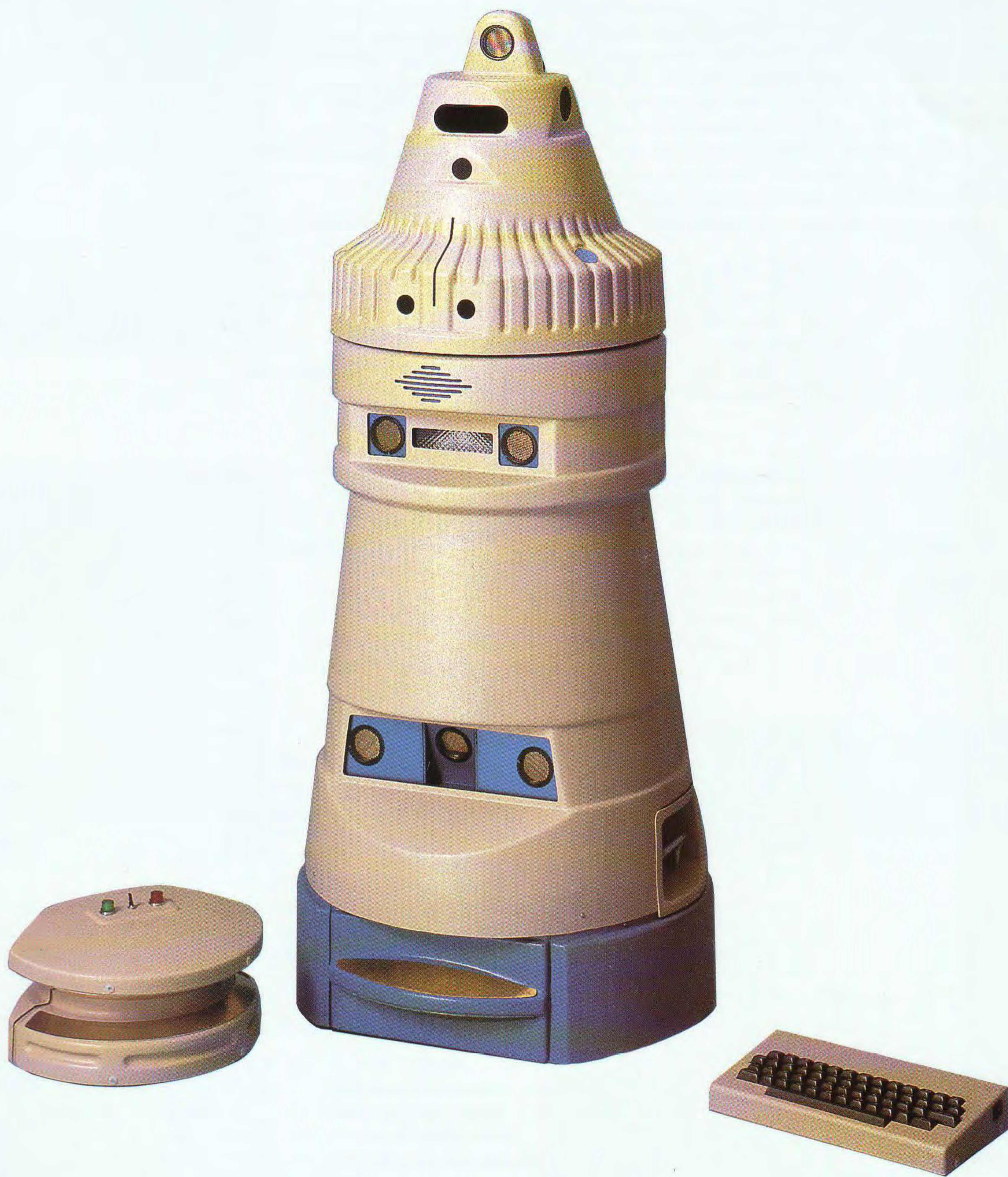
Front view of GEMINI showing sonars, lifelites, charging bumper, and three piece ABS plastic shell.
