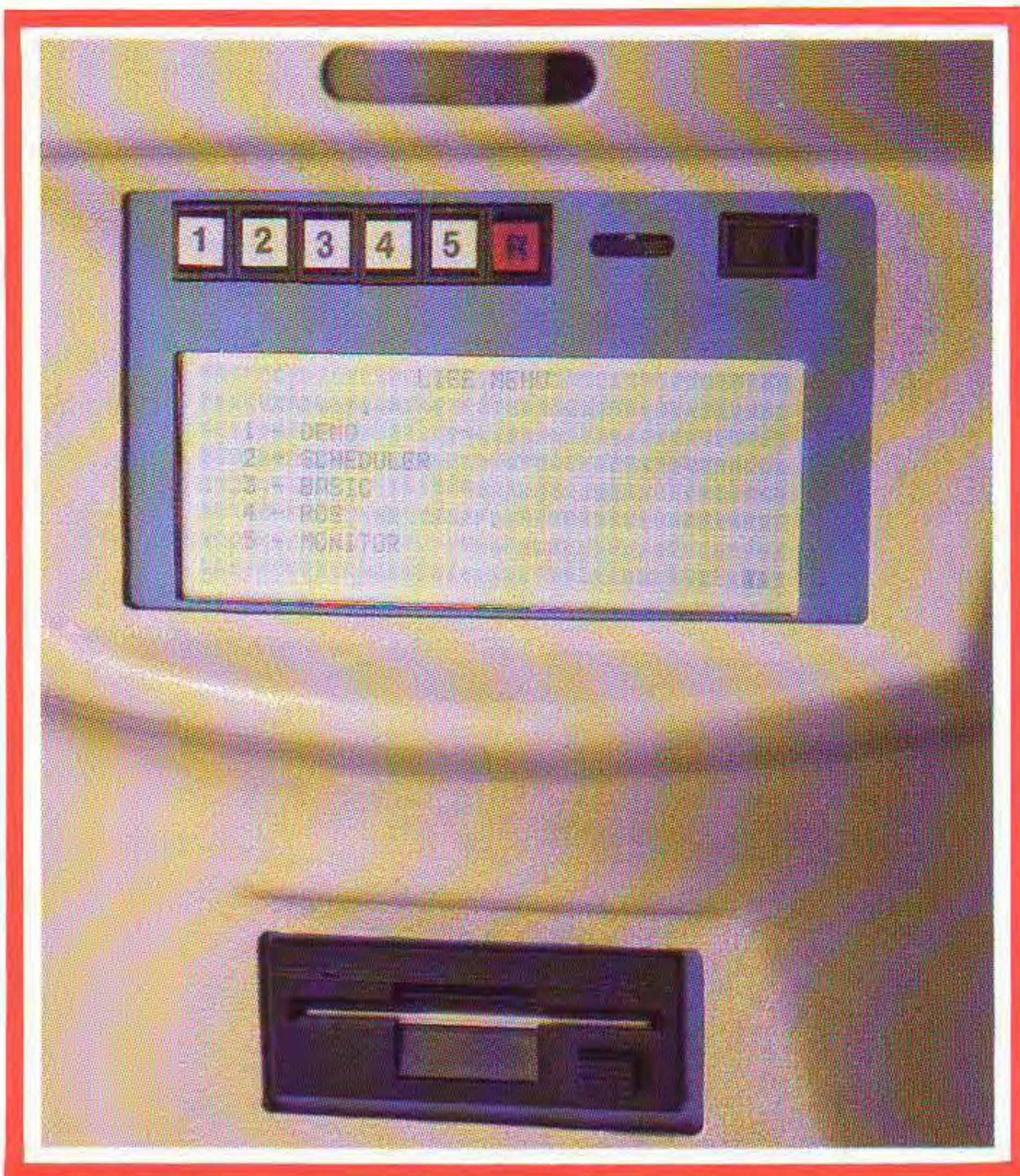
GEMINI's liquid crystal display with Life Menu. Above display is keyboard infrared receiver, below is optional disk drive.
