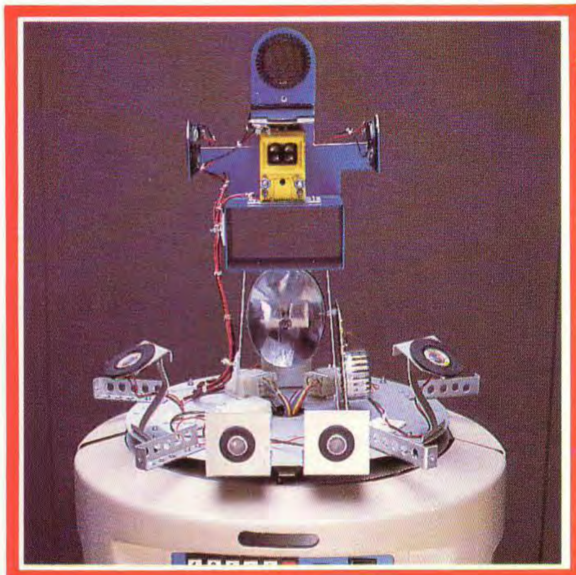
GEMINI's head contains sensors for motion and smoke, microphones for voice input and sound sensing, infrared room beacon and door edge detectors, ranging sonars, and room for additional peripherals.
