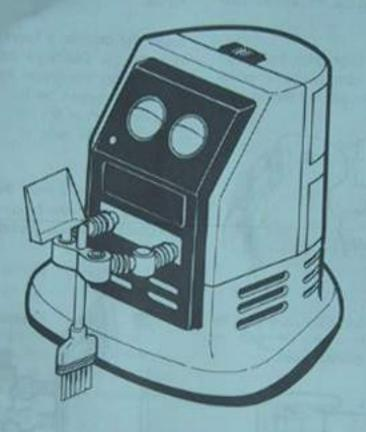
Your Radio Shack Dustbot sweeps and vacuums desks and tables. He detects the edge of a table or desk and automatically turns to avoid falling off.
